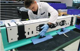
The ROHACELL<sup>®</sup> SHAPES department in Darmstadt, Germany supported the TUM Hyperloop Team with highly accurate CNC-shaped core parts. Through constant communication and excellent collaboration between TUM and ROHACELL<sup>®</sup> SHAPES, just-in-time delivery of the shaped cores to the TUM team meant they got the parts they needed at the exact time they were needed.
